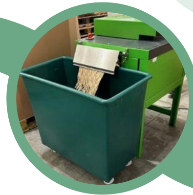
Cardboard is shredded onsite and turned into eco-friendly packaging material
